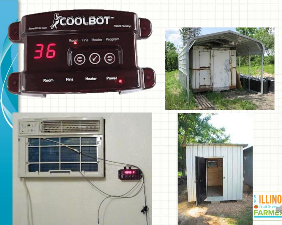
CoolBot systems take LONGER to cool down +CoolBot Systems recover SLOWER after you open the door +Poor functionality below 36 F (2 C) +You can't freeze things with a CoolBot +Running through the winter +Automatic Restart when you lose electricity
